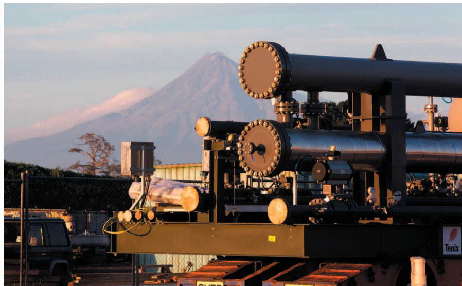
The 14m long, 4m width, 35-tonne LTS Skid for Greymouth Petroleum, LT separator, twin heat exchanger, piping and instrumentation fabricated by HERA member Tenix New Zealand at New Plymouth workshop. The scope of the Tenix contract included design to ASME VIII, AS1210, PD5500 Cat 1 TEMA R standards, all piping and instrumentation, protective coating system, and delivery to site
