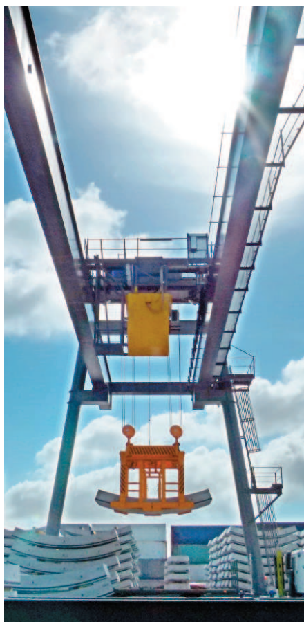
One of three 50t cranes fabricated by HERA member Baker Cranes lifting segments for Waterview Tunnel project
