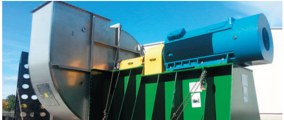
Polished stainless steel food grade dairy fan with 750kw motor designed and built by HERA member Windsor Engineering
