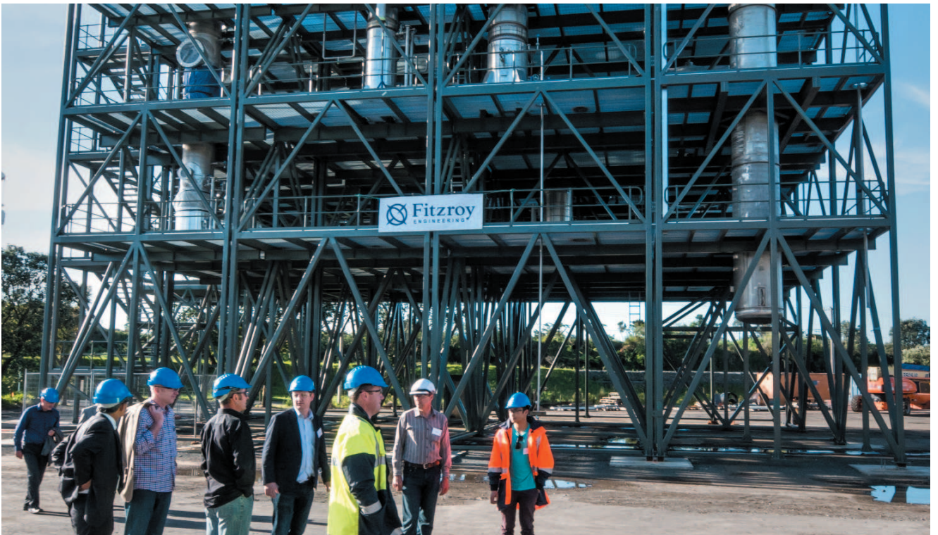
Visitors being shown around a oil recycling process module fabricated by HERA member Fitzroy Engineering Group in New Plymouth for Northern Oil Refining in the Queensland city of Gladstone. They will produce approximately 60 million litres of high quality hydrocarbon-based oils for re-blending and re-use
