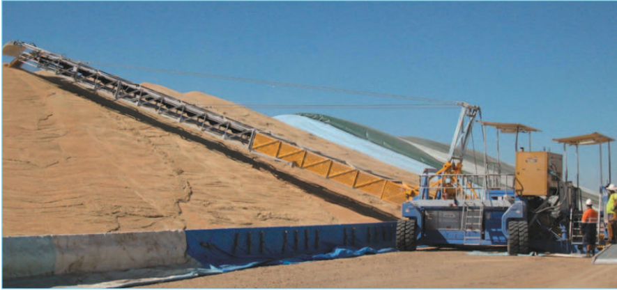
Development and manufacture of new generation mobile grain stacker by HERA member Southern Cross Engineering for Australian grain logistics company. The grainstacker is able to stack grain through a mobile device in excess of 750 tph. Traditional machines struggle to process 220tph.
