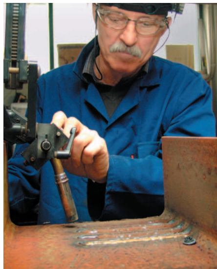
Senior Welding Engineer Alan McClintock performs welding trials to verify the effect of welding in k-areas of the rotary straightened I-beams
