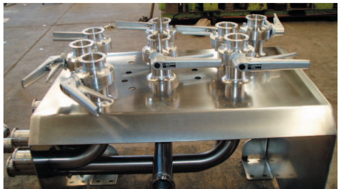
HERA member Stainless Engineering fabricated these stainless steel flow plates for export to the USA, making use of CNC profiling and bending
